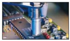
Open-circuits form a large category of manufacturing faults. The Q-Test technique is supported across the IFR ATE range. Developed and patented in-house, Q-Test detects open-circuits on custom or complex devices for which no access or data is available (for full test generation). Q-Test probes fitted to fixtures that incorporate a top-hat allow the technique to be fully exploited, cutting program development time and improving test coverage.
